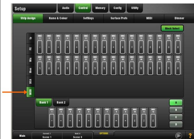
Each fader strip control can be assigned to transmit a custom MIDI message. This is ideal for controlling audio within a Digital Audio Workstation (DAW), a slave mixer, or parameters on external equipment such as effects devices. MIDI Strips can be named and coloured. They are stored within Scenes and can be made Safe from Scene recall.
