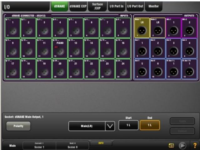
The panel background turns grey if the AudioRack is not connected. This means you can assign the sockets even if the rack is not plugged in.
