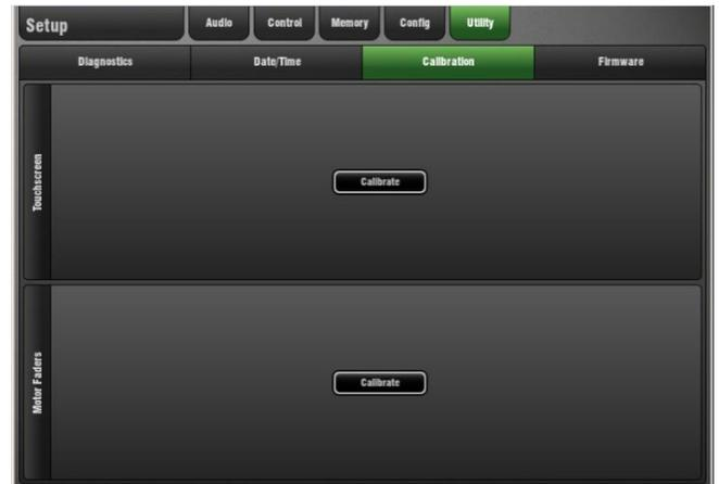
**To calibrate the Touch Screen** – Touch the Calibrate button. As accurately as you can touch the circle at the top left of the screen. Repeat for the other three corners.
