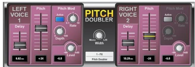
PitchDoubler is a stereo, pitch shifting doubler effect generating the effect of additional voices from its input. It is based on the same pitch shifting technology as VocalShift, with the associated low latency (<6ms), wide frequency range (down to around 80Hz) and minimal phasing / flutter artefacts. The effect squeezes two channels of high quality pitch shifting into a single effect slot, along with further features such as adjustable delay and modulation.
