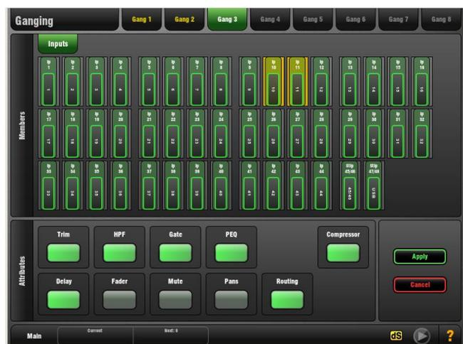
A Gang with channels already assigned highlights orange. Select either the Inputs or Mix tab. Touch the channels you wish to gang or ungang. Channels of a type different to those currently in a Gang disappear from the screen. Touch the parameters you wish to link in the Attributes pane. Adding the Routing attribute links the assignments and sends from the ganged channels.
