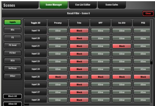
Touch the Recall Filter button in the **Scene Manager** page to open the filter window.
