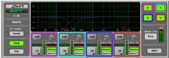
DynEQ4 is a model of the industry standard stereo 4-band Dynamic Equaliser. It is an advanced processing tool providing four bands of equalisation that respond to the dynamics of the signal.
