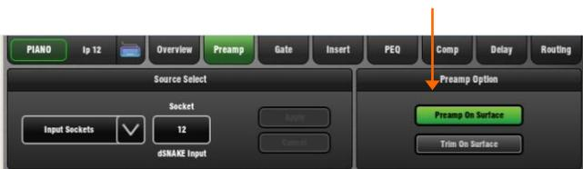
**Preamp on Surface** – The surface Preamp rotary adjusts Preamp Gain. This is the default for normal single console operation.
