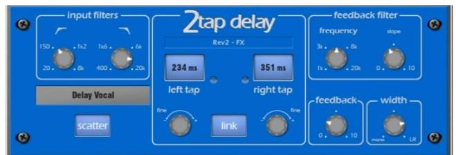
Separate left and right tap delay outputs from a mono'd input. Left and right delay can be dialled in using the screen Rotary, tapped on screen or tapped using a SoftKey. Individual tap indicators flash at the tap rate.
