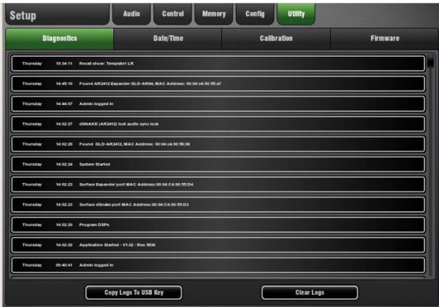
This keeps a timed log of events such as system boot up or shut down, and when Scenes or other memories were recalled. It also logs any errors recognised by the system.
