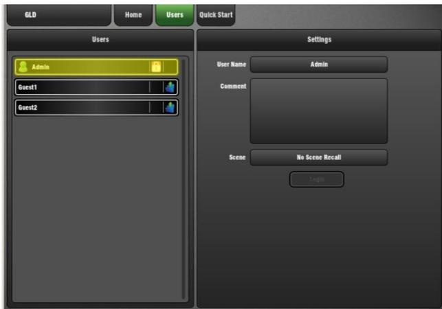
The system Administrator can set up to 9 User Profiles to protect settings and reduce operator error by restricting access to certain functions for different users.
