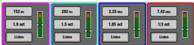
**Frequency control** - All 4 bands are full range 40Hz - 18kHz.
