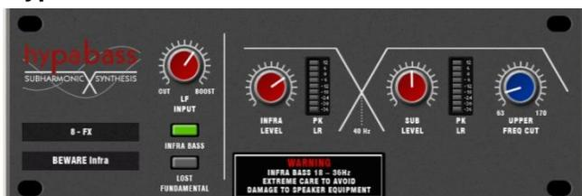
A sub-harmonic synthesis unit used in the live sound environment to generate infra and sub bass spectrum from weaker bass programme. We initially emulated the American analog classic, but implementation in DSP gave us the ability to use more sophisticated techniques in the sub harmonic generator and filtering stages. The result is reduced distortion in the infra bass section and much better independent control of the infra and sub bass spectrum, essential for live PA use.
