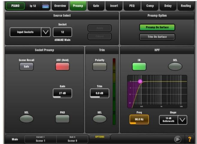
Touch a control box to highlight a parameter then turn the screen Rotary to adjust its value.
