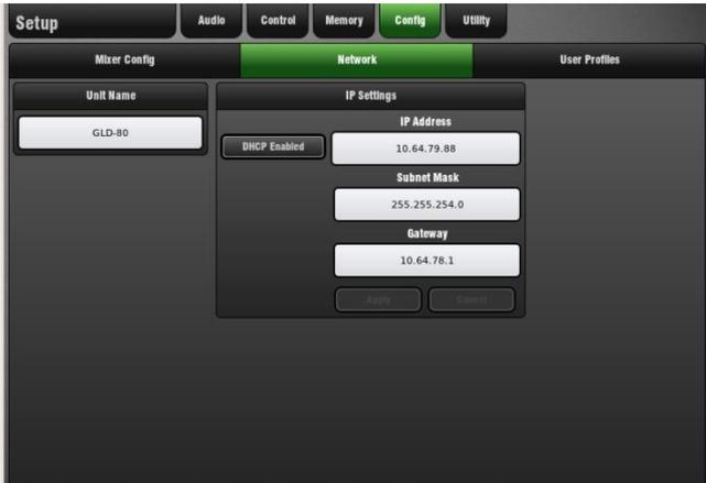
Some functions of the GLD can be controlled using TCP/IP messages via the Network port. The GLD TCP/IP protocol document can be downloaded from [www.allen-heath.com](http://www.allen-heath.com)
