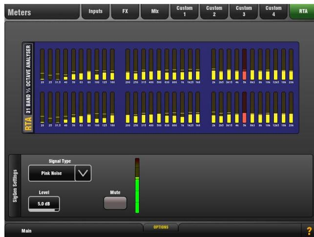
The RTA can be viewed in the **Home** or **Meters** screens. It also displays on the strip meters when GEQ Fader Flip is active. It separates the signal being listened to on the PAFL monitor into 31 frequency bands and shows the relative strength of each as a real time display.
