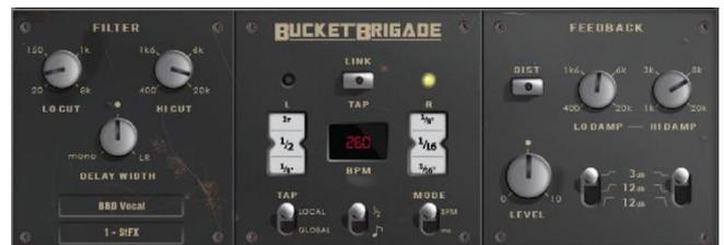
**MS mode** - The delay interval is set directly in milliseconds. The stereo beat delay can also be locked to the global tap tempo. There are controls for both input and feedback filters, with the latter having individual slope parameters.
