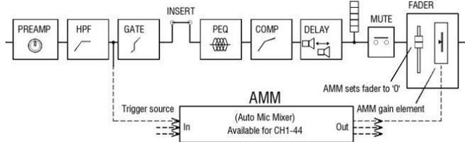
The AMM takes control by first setting each assigned channel fader to '0' (0dB unity gain), thus effectively passing the signal unaffected through the fader, and then using its own post-fade gain element to make its automatic adjustments. It is typical to leave the faders at '0', but they can be adjusted if the engineer wishes to make additional post AMM level changes manually to adjust the relative balance between mics in the mix.
