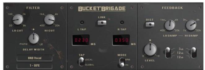
**Note** The Bucket Brigade Delay can also be locked to the global tap tempo. Global rate can be manually entered or tapped in using the screen of any delay FX locked to global tap tempo, or by tapping a SoftKey assigned as Global Tap Tempo.
