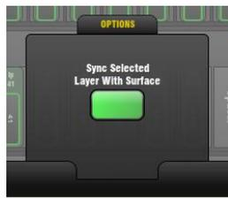
Use the pull-up to choose to sync the Layer shown on the screen with the currently selected surface Layer. Select the Bank to work with. The screen will follow the Layer currently selected on the surface for that Bank.
