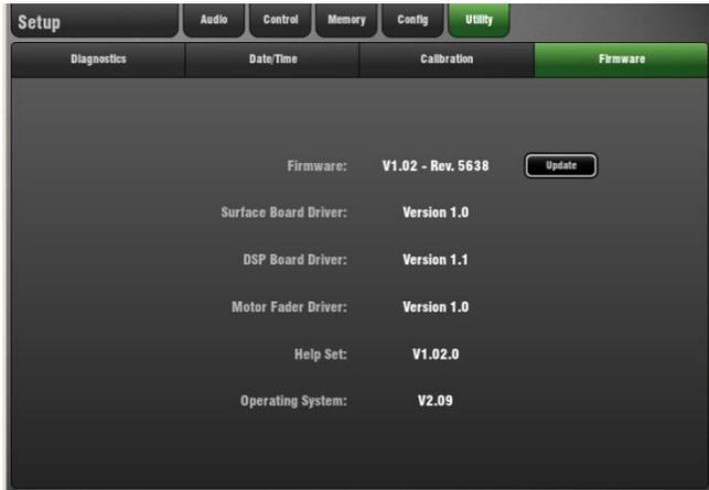
**To check the current Firmware versions** – You can view the GLD Firmware version on the **Home** screen or use the Firmware Setup page to view further details on the system firmware and other drivers within the GLD.
