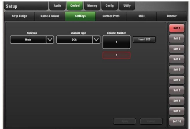
**To assign a SoftKey** -Touch one of the SoftKey buttons on the right of the screen to highlight it. Open the Function drop-down menu and select the function to assign. Use the Channel Type menu and Channel Number box to select the channel required. Touch **Apply** to accept, or **Cancel** to keep the current setting.
