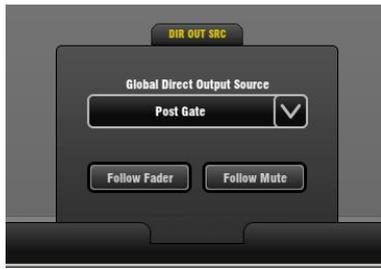
The global source for the input channel Direct Outputs can be set here using the drop-down menu. This setting affects all channel Direct Outputs:
