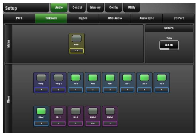
Use this page to assign Talkback to one or more of the Mix outputs. Touch a mix button to assign it On or Off.
