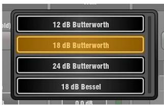
The filter can be switched in or out of circuit. A good starting point for vocal mics is to switch the HPF in and set to around 120Hz.
