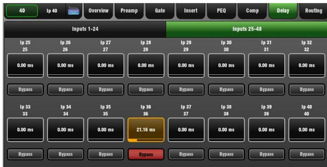
The currently selected channel is highlighted. Use the screen Rotary to change its value. Touch another parameter box to adjust the delay for a different channel.
