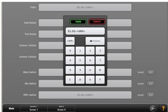
**Local** - Turn this button ON if you want the key indicator to follow local presses (toggle on/off by pressing the key at the surface). Turn this button OFF if you want the key indicator to follow remote messages (the MIDI device sends back a message to indicate current state). It is typical to set Local ON if you are using MIDI Strips to control a slave mixer. Set OFF if you are working with a DAW (Digital Audio Workstation).
