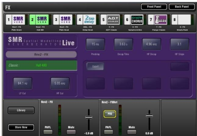
The **FX** Screen presents the 8 virtual rack slots shown across the top of the screen either empty or with FX devices already loaded. The FX name, current library loaded and metering is shown next to each icon.
