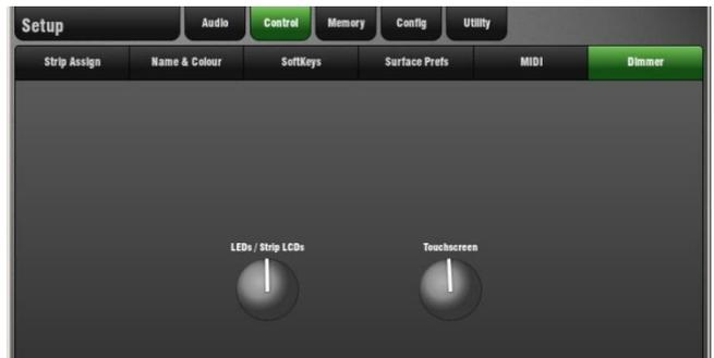
Pressing the **Setup** key for 2 seconds opens the Dimmer screen and sets the touch screen brightness to maximum.
