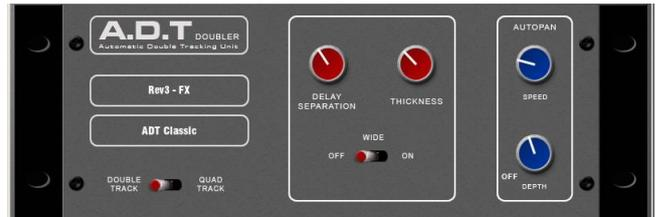
An Automatic Double Tracking module capable of creating short echo/chorusing, classic double tracking and 'slapback' tape delay loops.
