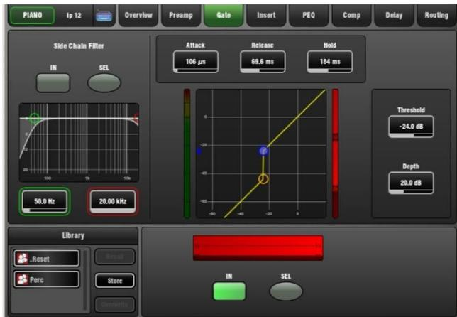
Touch and drag the curve or touch a parameter box. It highlights orange to show its value can be adjusted using the screen Rotary.
