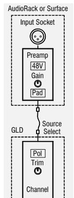
To provide a simple starting point the Template Show default is one-to-one mapping between input sockets and channels. For example, Socket 1 to Channel 1, Socket 2 to Channel 2 and so on.
