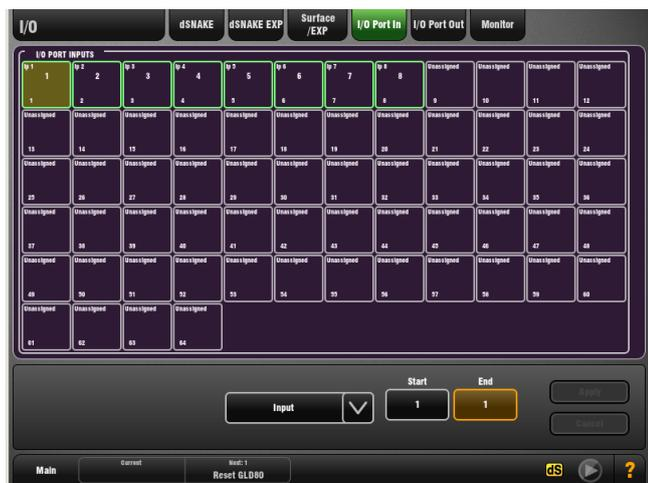
**GLD I/O Port** – Up to 64 channels of bi-directional audio via a digital audio network card fitted to the I/O Port slot. Various option cards are available from Allen & Heath, for example ACE, Dante, MADI, EtherSound, MMO.
