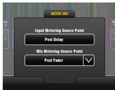
The meter source point can be globally set for all meters in the Mix page. This does not affect the fader strip or other screen metering.
