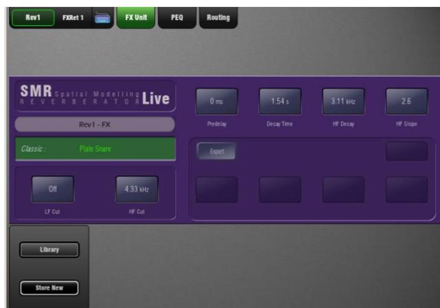
Touch the FX parameter controls and use the screen Rotary to adjust values. Touch a tab at the top of the screen to open the PEQ or routing window. The 4-band PEQ is available within the FX Return strip.
