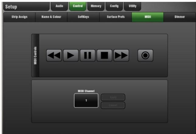
**To change the MIDI Channel** – Touch the MIDI Channel box. Turn the Rotary to select the required channel number. Touch **Apply** to accept or **Cancel** to leave unchanged.
