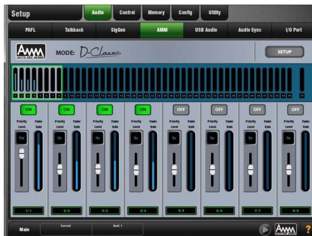
Unlike NOM mode which uses gating and fixed gain attenuation, D-Classic uses a 'constant gain sharing' algorithm to dynamically adjust the gain for each mic proportional to its input level. Louder signals will receive more gain in the mix.
