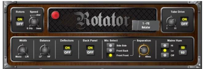
The Rotator is a model of a traditional rotary speaker cabinet such as those used to create the familiar Leslie organ sound. It simulates the rotating horn (treble) and woofer (bass) along with their crossovers.
