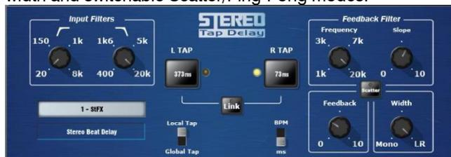
**Note** The Stereo Tap Delay can also be locked to the global tap tempo. Global rate can be manually entered or tapped in using the screen of any delay FX locked to global tap tempo, or by tapping a SoftKey assigned as Global Tap Tempo.
