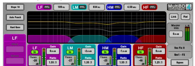
The Multiband Compressor can be loaded into one or more of the 8FX slots and then inserted into any of the input or mix channels.
