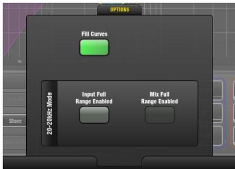
The frequency range for the 4 bands may be set globally for all inputs or mixes to be limited or full **20Hz to 20kHz**.
