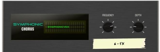
A faithful emulation of the 80's classic chorus effect. Simple to use and frequently requested. The unit has just two controls, Frequency and Depth, controlling the rate and delay range of the stereo modulator. The unit produces a rich, lively and wide chorus sound with a suggestion of very mild phasing / flanging.
