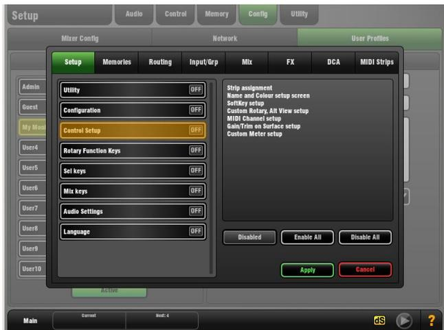
The Admin user can enable or disable access to GLD setup and mixing functions for guest users and operators. Each of the 9 other Users can have their own set of Permissions applied.
