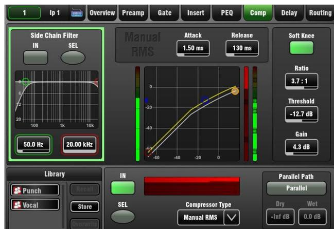
**Ratio** - Sets the amount of compression when the signal exceeds the threshold. A ratio of 1:1 means no compression. A good starting point for vocals is around 3:1. This means a 3dB rise in level at the input of the compressor would result in a 1dB rise at its output. To use the compressor as a **limiter** set the ratio to 'Infinity'.
