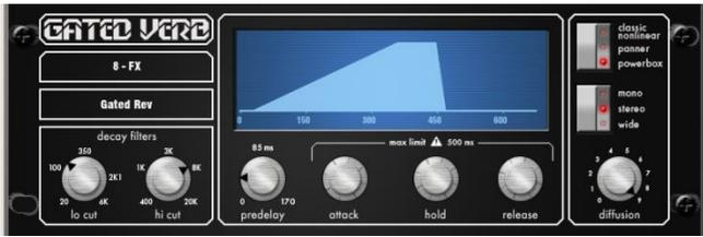
An accurate emulation of the classic 80's Gated Reverb plus two other variants called 'Panned' and 'Powerbox'. The user interface gives instant access to Lo-cut Hi-cut decay spectrum filters and the gate envelope controls - predelay, attack, hold and release.
