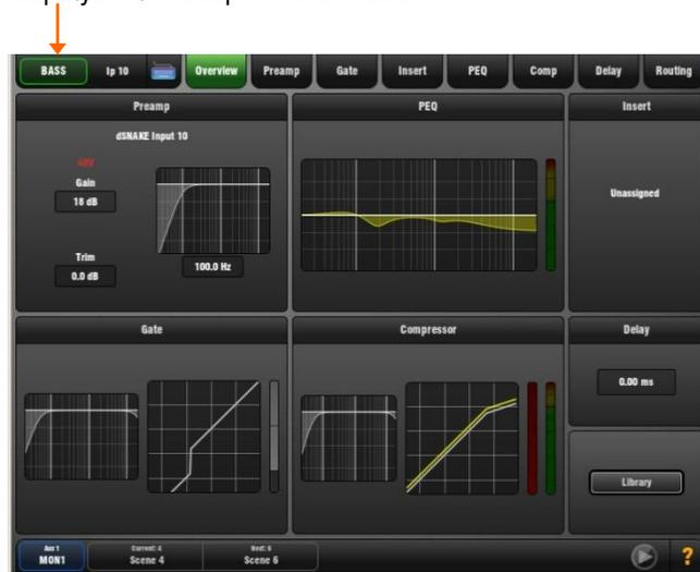
**Active Mix** – Displays the Name and Colour for the Mix currently selected using a fader strip Mix key is displayed at the bottom left of the screen. When the Main (LR) mix is active the status bar simply displays “Main”.
