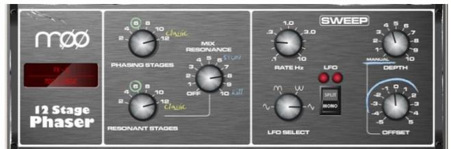
A classic 12 stage emulation producing rich textured phasing with plenty of control. The user has control of number of stages, feed forward and feed back, and ‘zero’ depth manual mode – to manually sweep the Phaser using the offset control.
