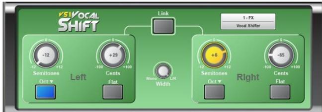
VocalShift VS1 is a stereo vocal pitch shifter squeezing two channels of high quality pitch shifting into a single effect. It has a very low latency (<6ms), covers the whole vocal frequency range, and minimises the phasing and flutter artefacts common with many pitch shifters.
