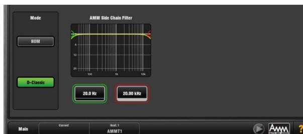
**Side Chain Filter** - Set High Pass and Low Pass filters to cut off frequencies below and above the normal speech range that may cause false triggering of the mics.
