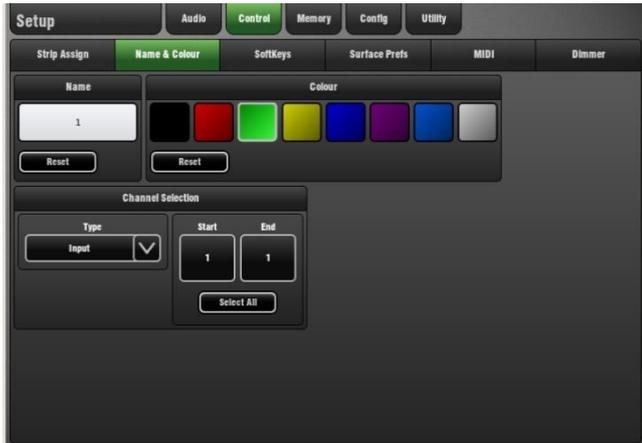
**To Colour a block of channels** - Select the channel type from the Type drop-down menu. Select All or touch the Start and End buttons to set the range of channels. Touch a colour button. This will change the colour of the block.
