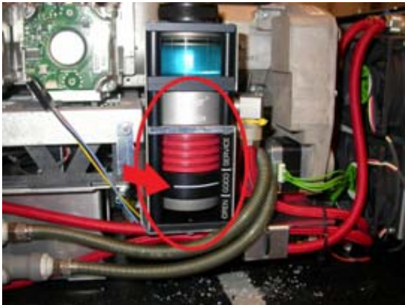
Image 15-1 Check cooling liquid
