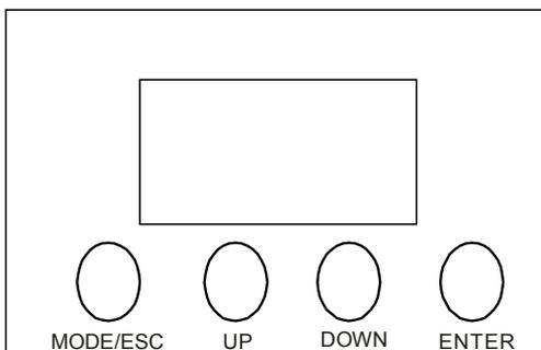
The main menu is accessed by pressing the Mode/Esc-button. Browse through the submenu by pressing Up or Down. Press the Enter-button in order to select the desired menu. You can change the selection by pressing Up or Down. Confirm every
