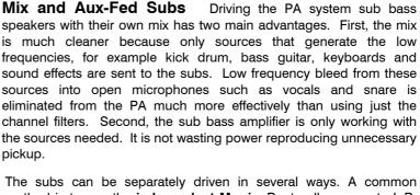
The subs can be separately driven in several ways. A common method is to use the **independent M mix**. Route all sources to L-R. Route the sources you want in the subs to both L-R and M. Feed the LR to a stereo crossover to drive the top speakers, and M to a mono crossover to drive the sub speakers. Refer to the speaker manufacturer for recommended crossover frequency, usually within the range 80Hz to 120Hz. The PA overall level is adjusted by moving the L, R and M (sub) master faders together.
