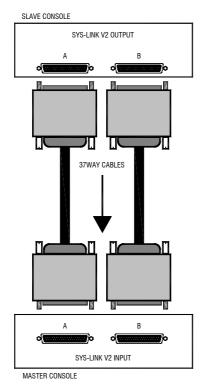
Sys-Link V2 input/output option A blank plate is fitted in both positions as standard. This may be replaced with optional cards which provide the console inputs, outputs and PFL system on pairs of 37way D connectors for linking to other Allen & Heath consoles already fitted with Sys-Link V2. The GL3800 can become an input channel expander (slave) or have its number of input channels expanded (master) when linked to other consoles.
