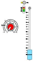
**Mixing with faders or gain controls?** There is a technique used by some operators where they set all the faders to '0' position and balance the mix using the channel gain controls. We do not advise this method as the signal to noise ratio and control resolution can be severely degraded. In addition, it is impossible to mix monitors from FOH in this way as changes to the gain settings affect the monitors too.
