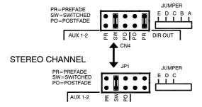
Channel Aux pre/post settings Factory default is Aux 1-4 = switched, Aux 5-8 = switched, Aux 9-10 = switched pre/post fader. You can change the setting of Aux 1-2 from switched to permanently pre-fade or post-fade if preferred. Make sure you set all mono and stereo channels the same. To avoid possible future confusion when the console is used by other operators, we recommend you only change these settings if absolutely necessary.
