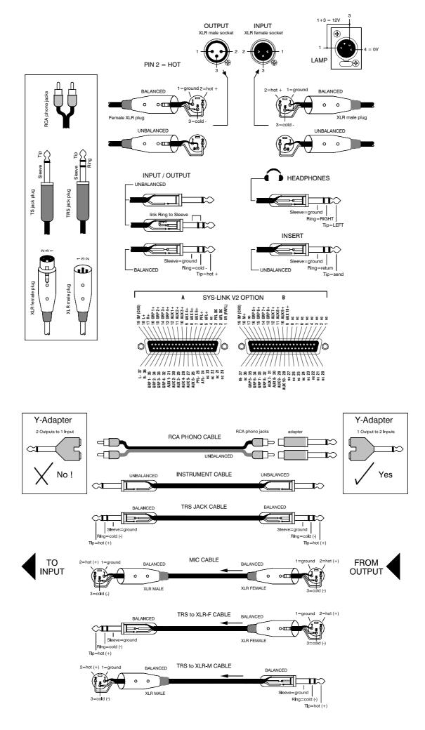
The GL3800 uses professional grade 3 pin XLR and 1/4" TRS (3 pole) jack sockets. To ensure best performance, we recommend that you use high quality audio cables and connectors, and take time to check for reliable and accurate cable assembly. It is well known that most audio system problems are due to faulty or sub standard interconnecting leads. The following plugs may be used to connect audio to the console:
