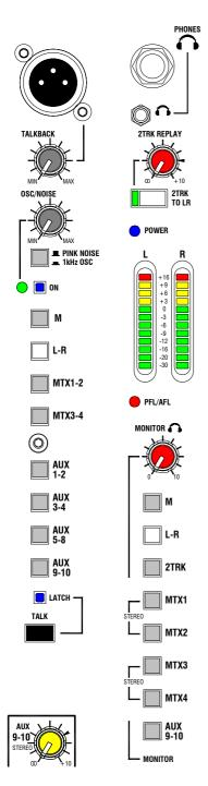
**2TRK REPLAY** A stereo source such as a recording playback or walk-in CD can be routed directly to the main LR mix. Adjust its level from fully off to +10dB gain using the rotary control. You can check the source on the meters and in the headphones before bringing it into the mix by selecting the 2TRK monitor switch.
