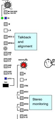
**Applications for the Matrix** The matrix is a 'mixer within a mixer', a versatile toolbox of outputs you can use to satisfy a host of applications. Each of the 4 outputs is mixed from any combination of the groups, L, R, M and an external input as dialled up on the 12 source rotaries (hence a '12x4' matrix). Its master level can be adjusted independently. Using combinations of the outputs you can create mono, stereo or multiple output mixes. Some applications include:
