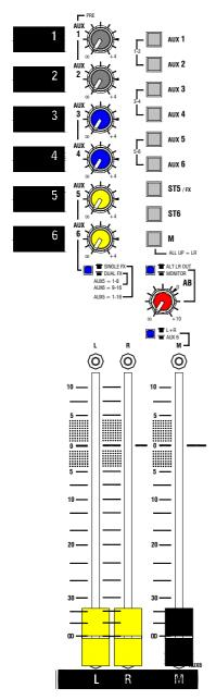
**AUX MASTERS** Each aux mix has a master level control that adjusts the output level to match external equipment, or to trim the monitor, effect or other send without affecting the mix balance. Up to +4dB boost is available above the normal 0dB position.
